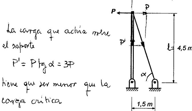
$$P_{cr} = \frac{M^2 E I_z}{l^2} = \frac{\pi^2 \times 200 \times 10^9 \times I_z}{4,5^2} > 3 \times 600 \times 9,8 \\ = 17640 \text{ N}$$
