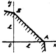
$$\begin{cases} \sigma_{xx} = \frac{\partial^2 \phi}{\partial y^2} = 6x + 6y \\ \sigma_{yy} = \frac{\partial^2 \phi}{\partial x^2} = 6x + 6y \\ \tau_{xy} = -\frac{\partial^2 \phi}{\partial x \partial y} = -6x - 6y \end{cases}$$
